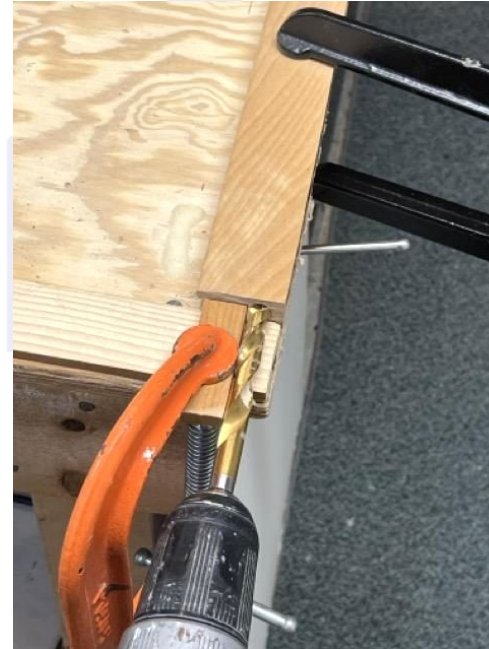
Drilling tube holes with the bit parallel to the guide block and to the table top
